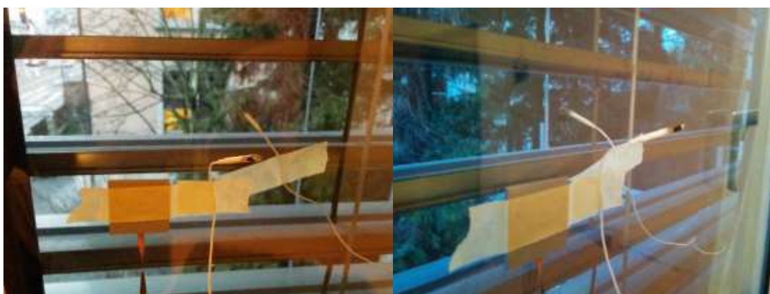
Figure 1: Measurement set-up: Window with metal exterior shutters; Heat flux sensor with 2 temperature sensors, one inside and one outside, both roughly 2 cm away from the glass.
