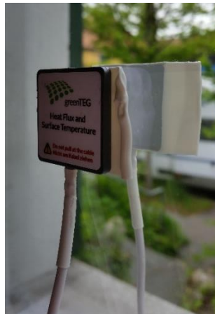
Fig. 2: Window glass with sensors on both surfaces.
