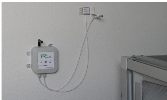
Fig. 4: gOMS sensors for measuring heat flux, surface and room air temperature on the inside wall of office B5
