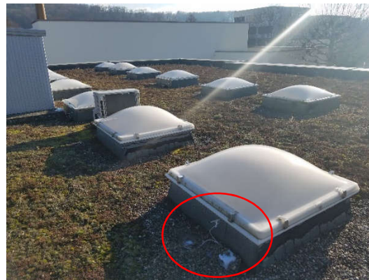
Figure 3 Nodes placed on the north-facing side of the skylight to avoid radiation exposure
