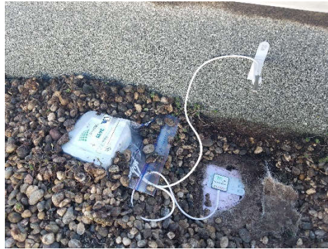
Figure 4 Protecting nodes from water ingress using Ziploc-like plastic bags and removing gravel until a flat and clean surface was reached
