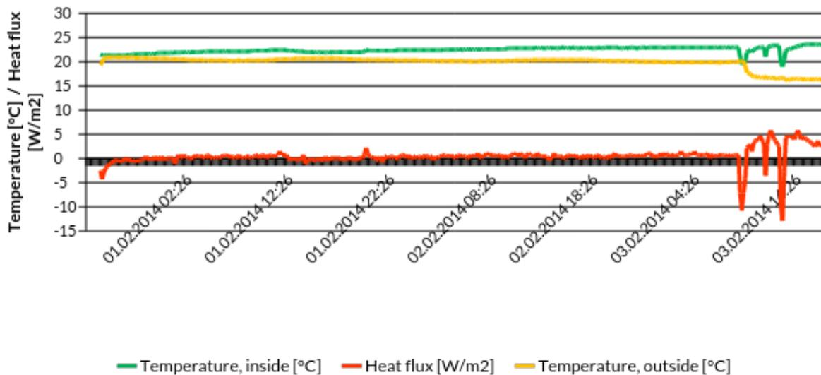
Figure 5. Temperature and heat flux graph of spot B. The outside temperature corresponds to the temperature in the cellar. This graph was created using the (old) software included in the measurement device (new software version shows directly U-value graph).
