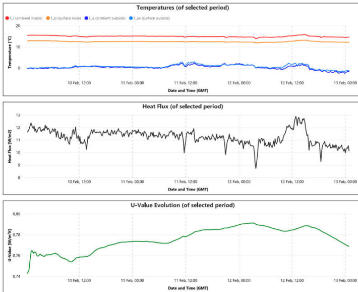
Figure 4.1-1: U-value measurement data of the uninsulated wall
