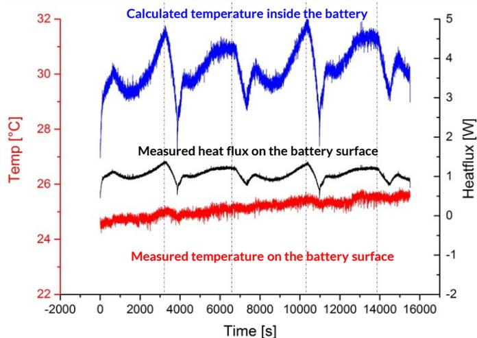
Heat flux (black) and temperature response (red) measured at the battery surface. The temperature inside the battery (blue) is determined by knowing the heat capacity and thermal resistance of the battery
