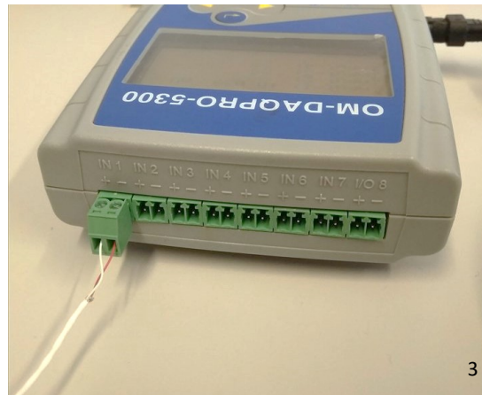
Figure 2. 1,2 show how to connect the cables to the terminal and 3 how to plug it back to the socket
