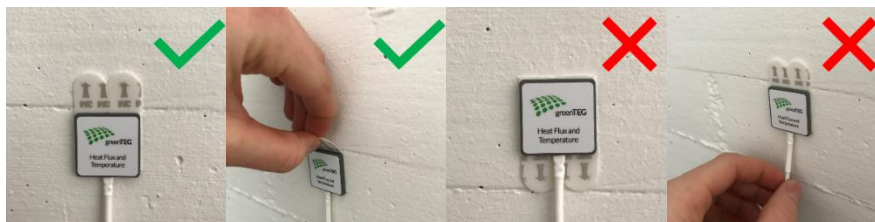
Figure 2 How to correctly mount and detach the sensor (left) and how to do it incorrectly (right).
